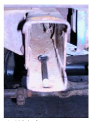
1. With frame exposed, place the nut over the back hole.
