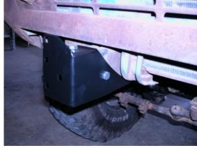
2. With tab in place, install bracket over frame as shown (opposite for other side). Using supplied flat washers and 1/2" bolts, install top, inner, and the two lower bolts (4 total). Snug but save final tightening until after the bumper has been installed and adjusted.
